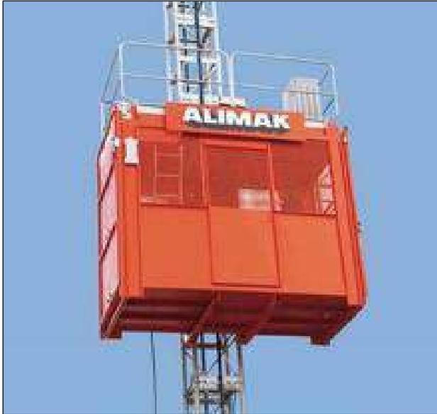
**Figure 16-32: Alimakhek Scando 650 Construction Man Hoist**
