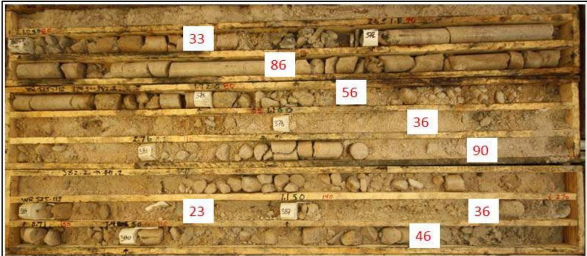
**Figure 16-9: Poor to Very Poor Rock Mass Conditions in the Broken Zone Domain (% Core Recovery Shown)**
