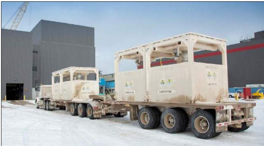
**Figure 17-3: B-Train Tractor Trailer with Special Slurry Containers**
