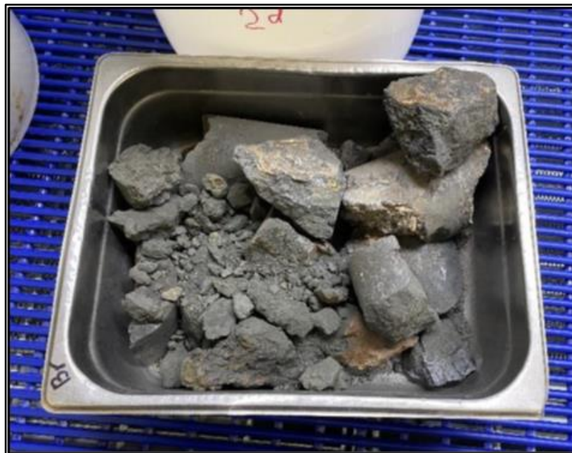
Figure 13-4: HGU 2d: Column Leach Test Composite. Prior to Crushing and Screening. Dense, Moderately Friable, Hematite Cement
