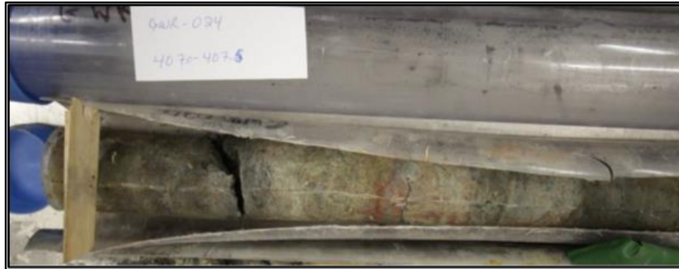
Figure 13-5: HGU 2e: GWR-024, 407.50 to 407.70 m – Lower Clay Zone Moderately Friable, Altered Grey Clay, Some Hematite
