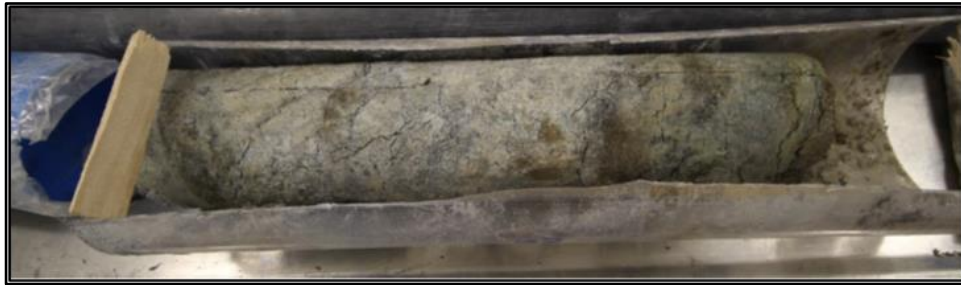
Figure 13-1: HGU 2a: GWR-022, 404.40 to 405.90 m – Soft, Friable, Altered Grey Clay, Pockets of Uranium Mineralization Disseminated
