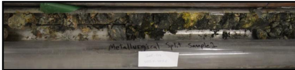
Figure 13-3: HGU 2c: GWR-016, 405.50 to 407.00 m – Rubble, Friable, Red Redox Fronts, Yellow and Grey Pockets
