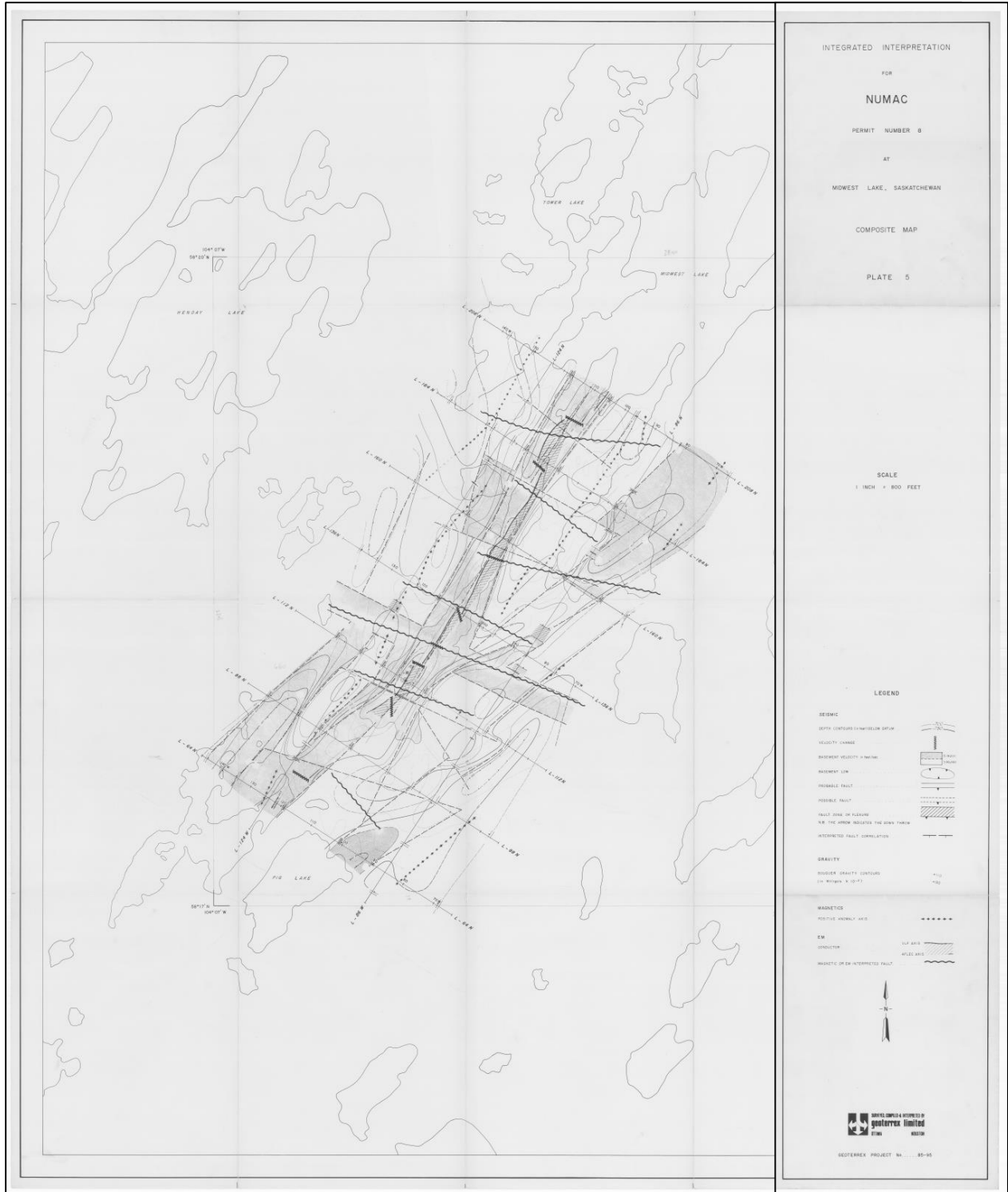
Figure 9-1: Composite map of geophysical interpretation of seismic, gravity, magnetics and EM results (GEOTERREX, 1970)
